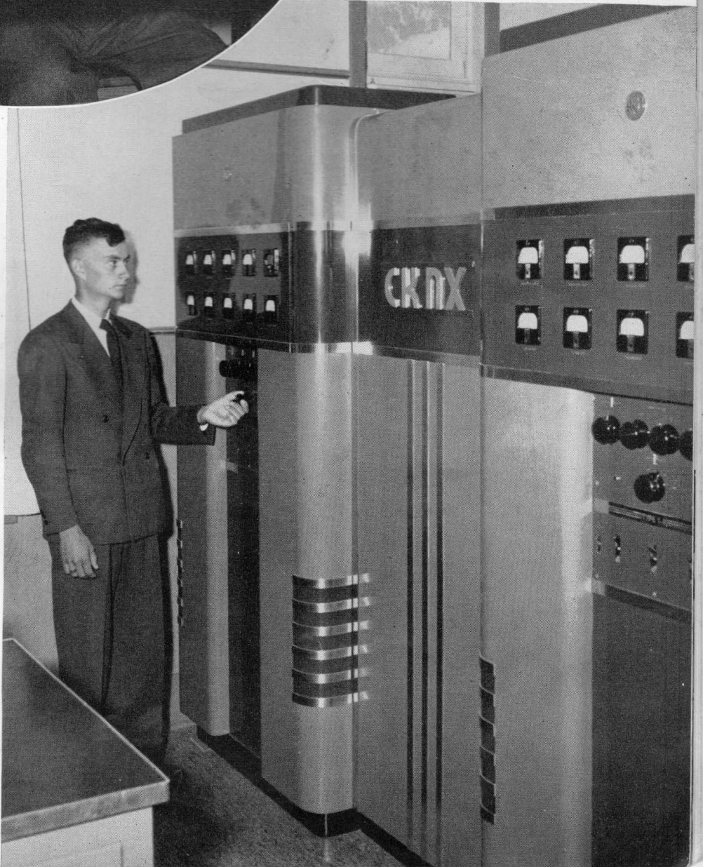
Operator Jack Salter checks performance of 1000 Watt transmitter.
